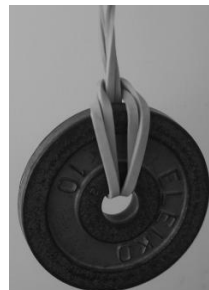
Figure 1: Suspension of a 10kg metal disc in the rubber band in order to create an unstable load.
