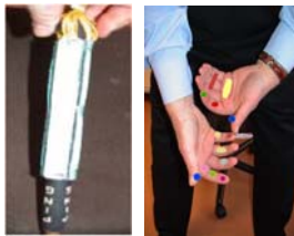
Figure 1: Pressure sensors at the grasp of the golf club (left) Analyzed pressure areas at the left and right hand (right)
