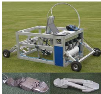
Figure 1: TrakTester (at the top) an, adjustable (bottom left) inflexible foot models (bottom right)
