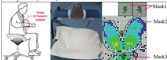
Figure 2: Ergonomic chair with chest support (left), pressure measuring system (center), masking contact area (right)
