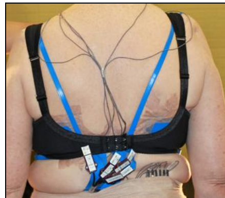
Figure 1: Measuring pressure exerted by the bra band, strap and cup of a breast cancer survivor.
