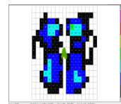
Figure 2: Avg pressure map of pad with raised gel points. High pressure areas are located along the gel points.
