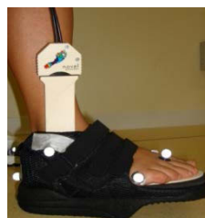
Figure 1: The WPS® talus shoe (Podartis, Treviso Italy) with a talus outsole equipped for the biomechanical evaluation.
