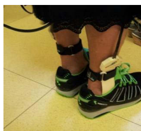
Figure 1: Biomechanical shoes with Pedar insole system for baropodometric evaluation.
