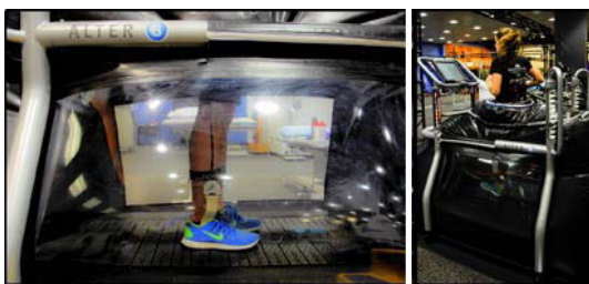
Figure 1. The initial set-up of the pressure distribution measurement insoles on the PPT.
