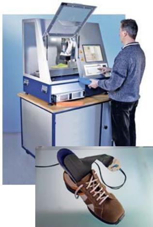
6. Prove pressure reduction of the footwear by measuring inside the shoe with a pedar<sup>®</sup> in-shoe pressure measuring system during normal free gait in repeated steps.
