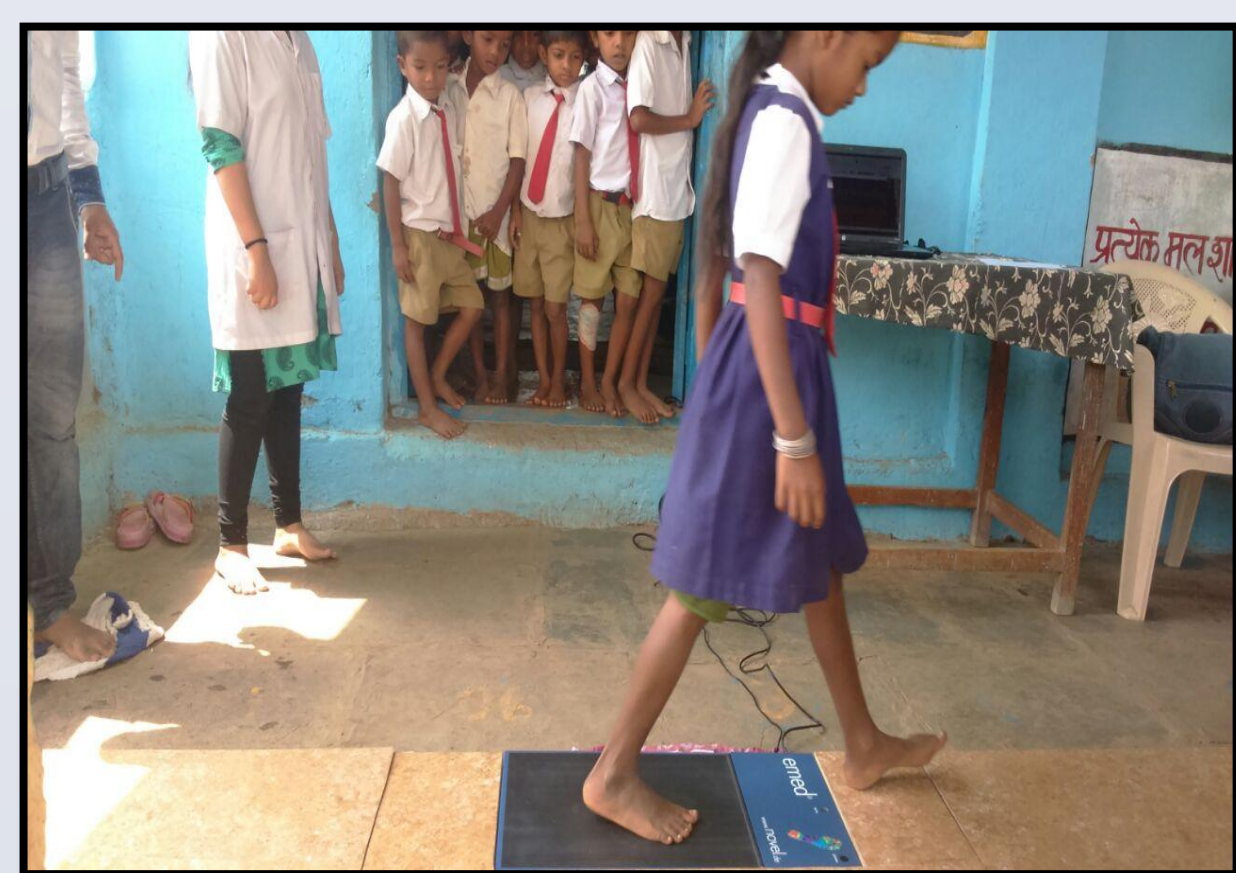
Figure 1: Use of emed-sf system to record foot pressures and foot geometry
