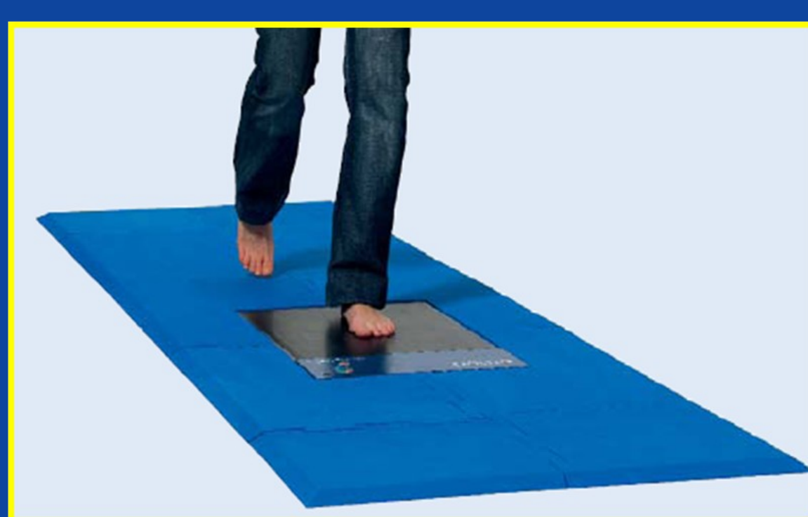
Figure 2. An example of the measurement of dynamic arch index by using emed-at2 platform.
